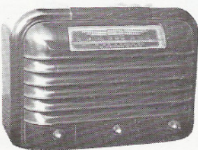
Ultimate model RU, 5-valve BC 1947. The bakelite cabinet was the largest made in N.Z. at that time.
