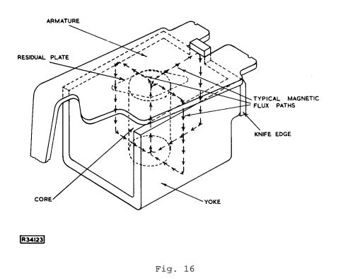
The electromagnets of the Type 1 Uniselectors give an insufficient margin of power with heavy wiper loads, so a more powerful electromagnet system has been designed for the Type 2 and 3 Uniselector. A single coil is used, wound on a large diameter core and fixed in a box-shaped yoke, with the armature completing the magnetic circuit as shown in Fig. 16.
